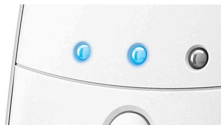
Lights are activated to indicate the level of sound in your baby's room, even when the Parent Unit is muted.
